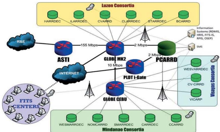
Figure 5. The current network configuration of PCARRD
