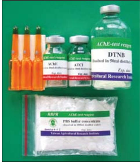
**Fig. 14.** The kit for pesticide detection of AChE
