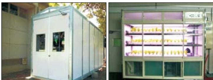
*Two mobile types of plant factory, a two-compartment model growing lettuce and mushroom simultaneously in the same container (left) and a simply equipped model growing one single crop as a store showcase (right)*
