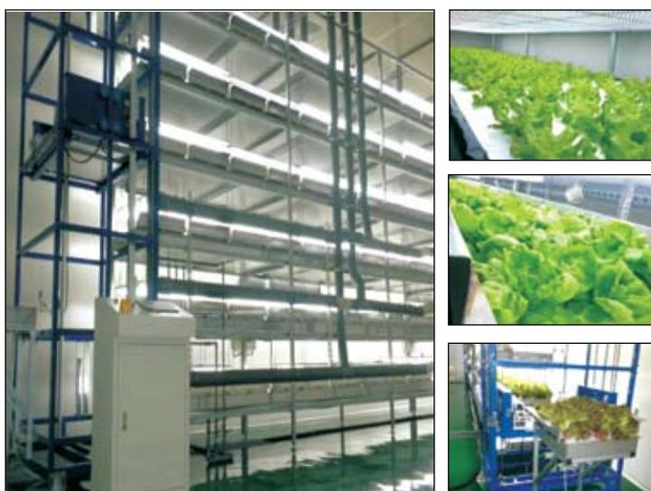
*High-performance three-dimensional modular shelving system using artificial light source for a re-circulating water culture method*
