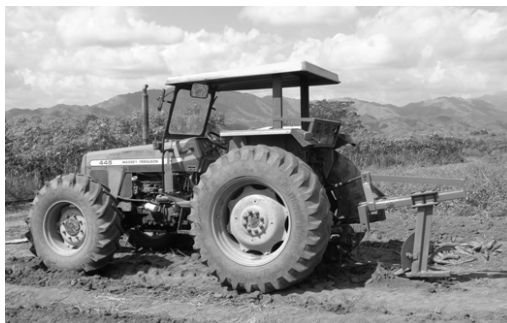
Figure 4. Cassava digger prototype with sturdier frame.
